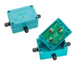
The FG-DCTL addressable box allows the connection of one analog sense cable (1 to 45m, "cut to length") to the main bus wire from the digital panel. FG-DCTL will create an 45m address on the panel for that sense cable.
