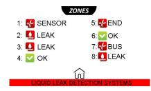
The "home" button allows to back to the main page. It displays the lengths or change the MODBUS. The system will come back to the "home" screen after 30 seconds of inactivity.
